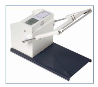
Quality Mixer is a new fully automatic mixer/tube stripper manufactured to simplify and standardise the requirements of QC according to Directive 2004/33/EC, Article 6 Appendix V2
